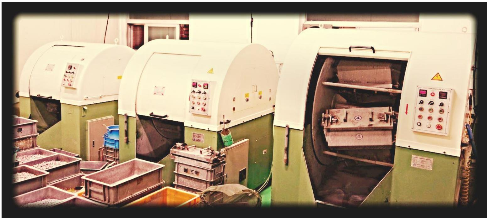
The barrel grinding team uses computer programmed rotating machines to guarantee that each item is polished to a high standard (sharp and rough edges are made smooth in the tumbling machines).
